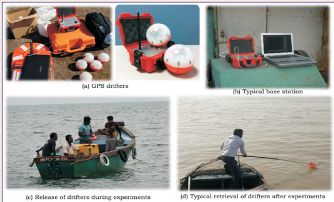
Fig. 5 GPS drifters, typical deployment and retrieval
