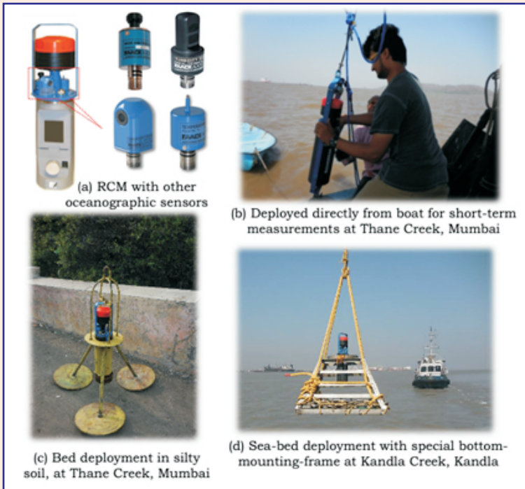
Fig. 1 RCM and installation methods
