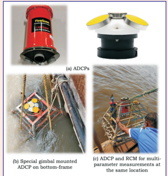
Fig. 2 ADCP and typical deployments
